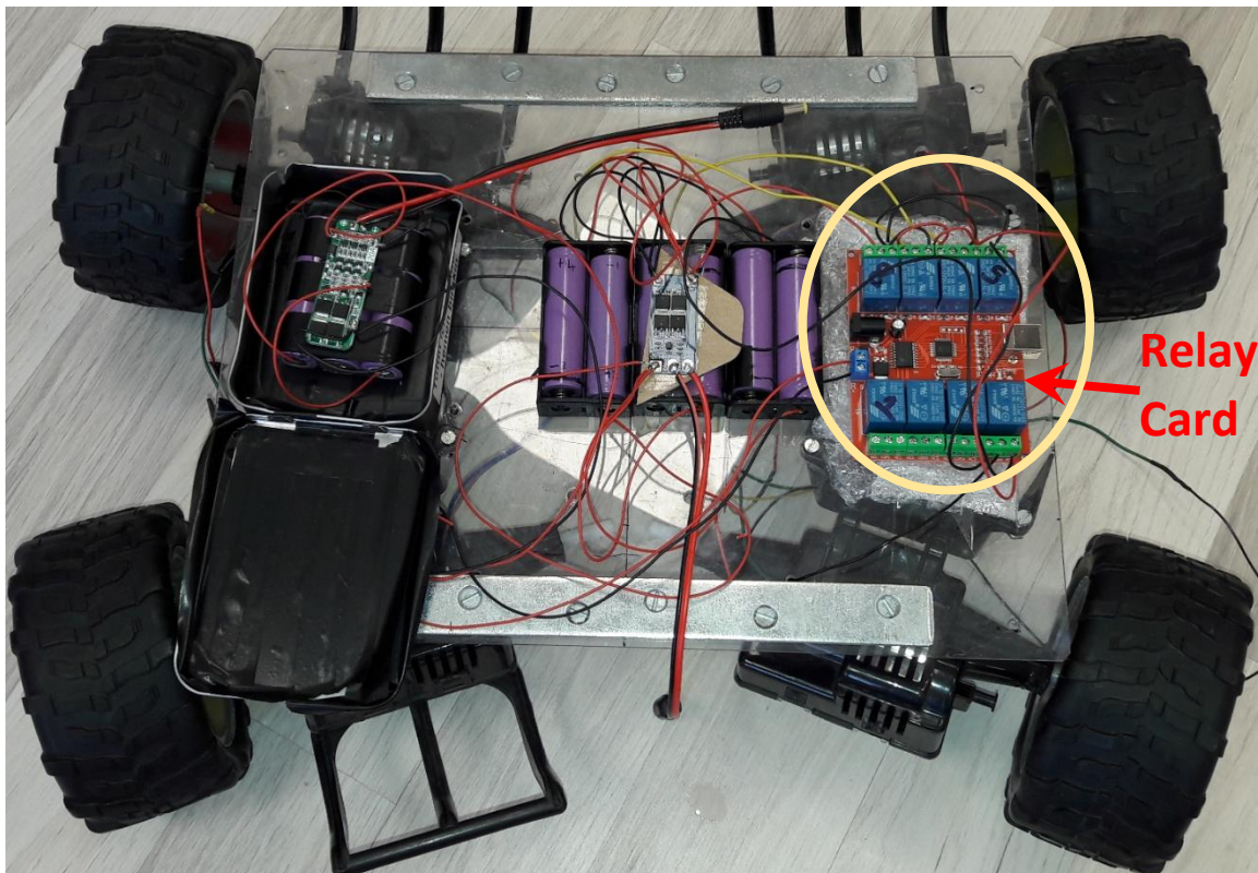
Figure 4.2. Inside of a 4-wheel drive mobile robot. The encircled electronic card is a DCTTech 8 channel USB relay card. Tiny blue boxes on the card are the relays.
